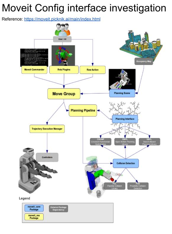
MOVEIT2 package gives more capability and functionality for serial manipulators Based on Figure 1. We need to develop or outsource the grey rectangles these are dependencies that need to be met: PCD, FCL, CHOMP, OMPL, SBPL And the controllers.
